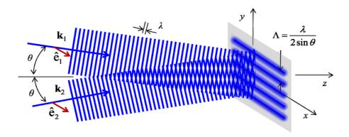
Figure 3: Two-beam interference with different incident angle. This figure is in the reference [2].
