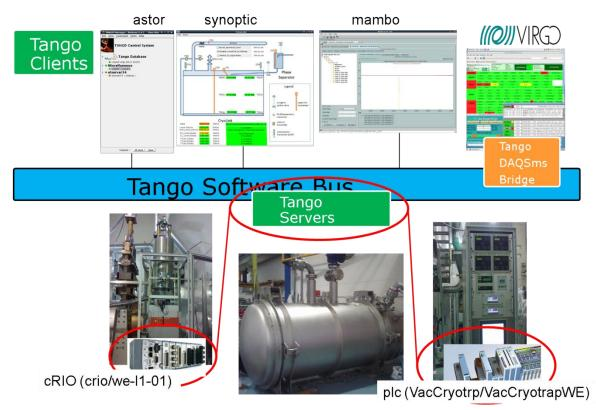
Figure 2 Tango Clients and Servers for the cryotrap control at west-end
