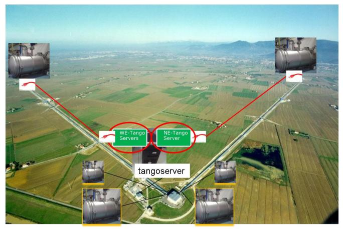
Figure 1 Large cryotraps controlled by tango servers
