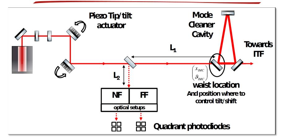
The Near Field (NF) and Far Field (FF) optical setups will be designed to optimize and decouple the sensing. Near Field and Far Field QPDs will sense the shift and the M.Mantovani LVC Nice 18/03/14 tilt at the IMC input ( $x_{IMC}$ ,  $\mathcal{G}_{IMC}$ ) respectively.
