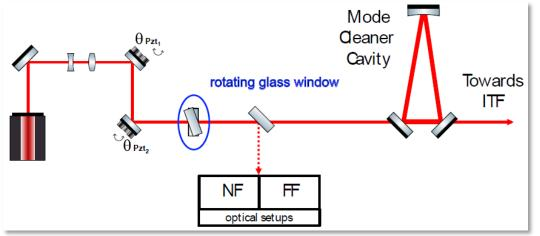
The two quadrant signals decoupling can be easily evaluated by inserting and rotating a glass window to purely shift the beam at the Input Mode Cleaner input.
