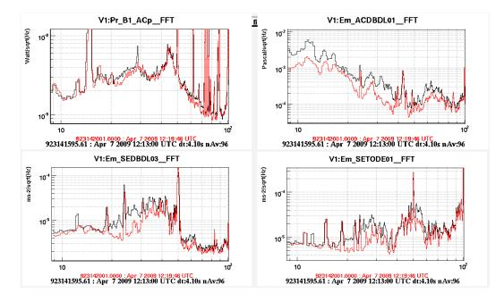
**Figure 4.** Effect of switching off the CB hall HVAC machine (April 2009): black curves correspond to the machine ON, red curves are with machine OFF. Upper left plot is the dark fringe, Upper right is the microphone on EDB, Bottom left is one seismometer on EDB and Bottom right is one seismometer on DET tower output window.
