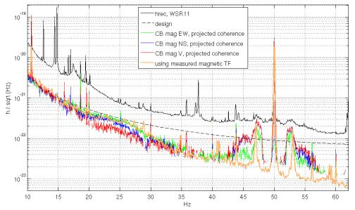
**Figure 13.** Projection of magnetic environmental noise coupling to mirror magnets in the central experimental hall. WSR11 data. The noise around 50Hz is due to the switching heating resistance of the MC building HVAC, as explained in Sec. 4.1 item (4).
