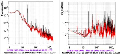
**Figure 10.** Acoustic and seismic noise produced by the vacuum scroll pump serving the DET tower. Black curves are with pump on, red curves with pump off. Left plot is a microphone on the EDB, right plot is a seismometer on the DET tower output window.
