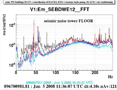
**Figure 12.** Seismic noise of WE hall floor produced by the air conditioning (black to red), the vacuum pump (red to blue) and the racks (blue to cyan). Measurements are partially limited by sensor noise.
