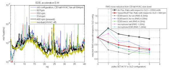
**Figure 3.** Measured reduction of a seismic noise (LEFT) on EDB consequent to the slow down of fans of the Central hall air conditioning. Residual noise is the difference of black and yellow curves. (RIGHT) RMS noise reduction of seismic and acoustic noise in CB hall and Detection, as function of the air flux and speed of HVAC inlet fan.
