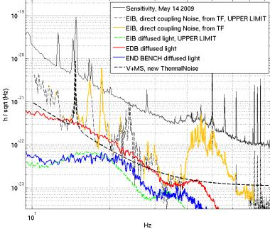
**Figure 5.** (TOP) Projection of environmental noise coupling through motion of external benches, as of April 2009. (RIGHT) Tentative projection of the same noises for V+MS.
