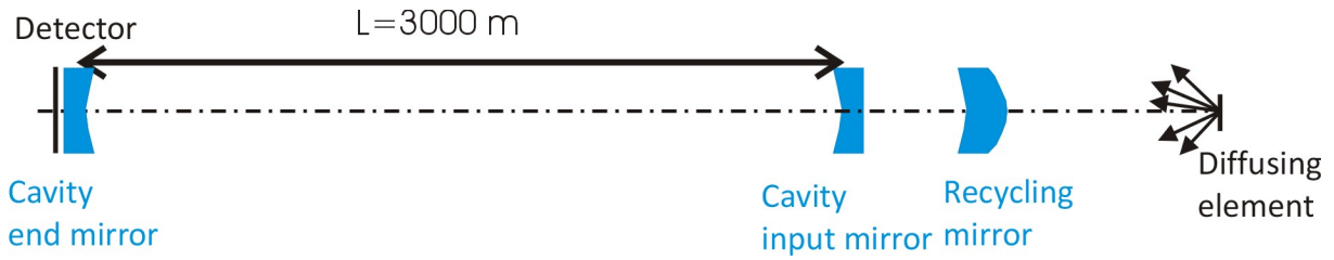
Figure 28: Setup considered for the comparison of the two calculation methods. The light emitted from a diffusing element located after the PR mirror is considered recombined if it reaches the end mirror.
