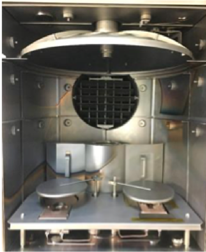
Figure 6: Upgraded OptoTech OAC-75-RF coater with dual e-gun configuration
