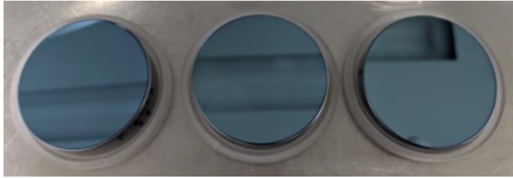
Figure 8: Optically equivalent coatings on 2" Si substrates. The coating on the left was made before the addition of the second e-gun. The middle and right coatings are far better optical matches
