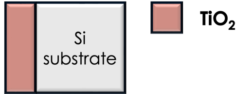
Figure 21: Schematic of TiO_2 layer on Si substrate.
